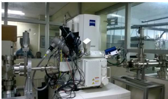
Figure 3: Advanced irradiation cum FESEM imaging Facility.
