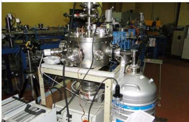
Fig. 4b PIGE facility at FOTIA with scattering chamber and HPGe detector
