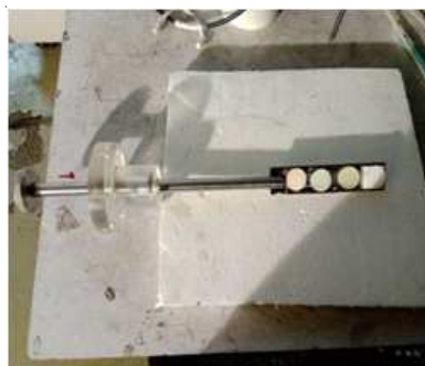
Fig.2: Target pellets (20 mm diameter and 2 mm thick) mounted in the SS sample ladder
