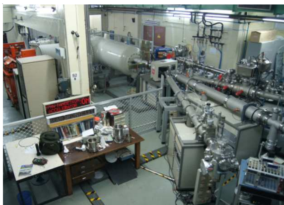
Figure 1: 1.7 MV tandatron accelerator with its beamlines
