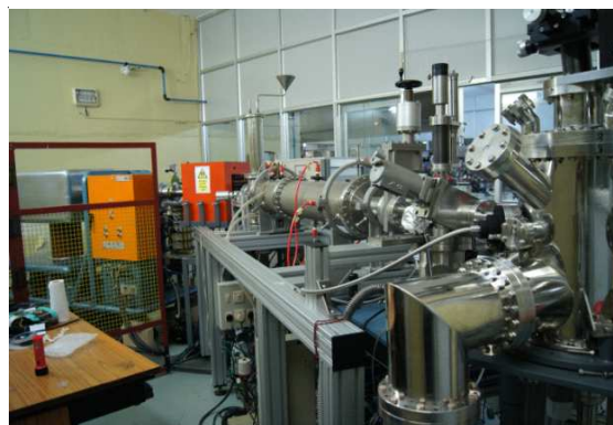
Figure 6: 150kV Gaseous ion accelerator.
